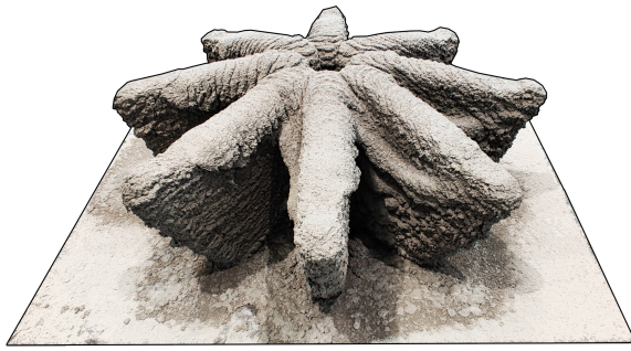
Figure 6. Column capital printed with printing interruption routine
